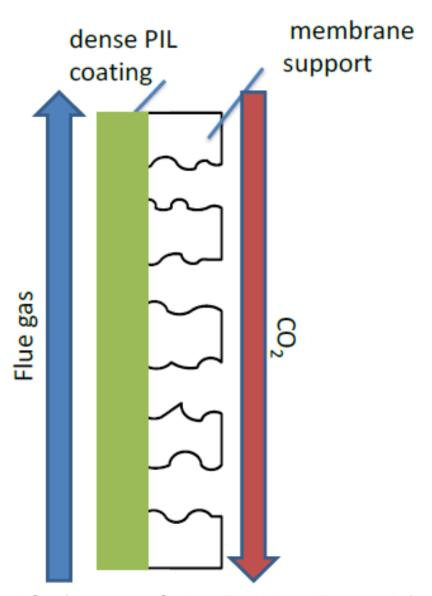
Conceptual scheme of PILs used in dense gas membrane
